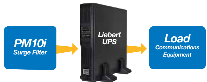
Liebert GXT3-2000VA UPS installed in a local rack unit to protect sensitive communications equipment
